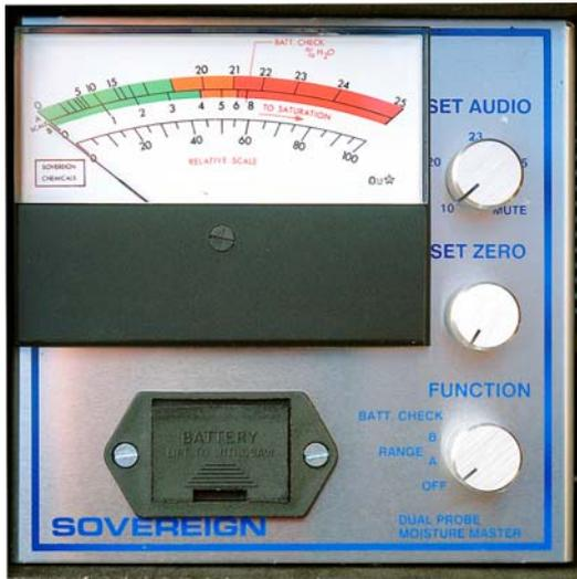
The Sovereign should be set to 'Scale A' regardless of whether the vessel is kept in salt or fresh water. If possible, switch the instrument on a few minutes before it is required to allow stabilization.
