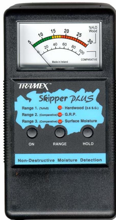
If an osmosis prevention or treatment is to be carried out, readings must be lower than 14% H<sub>2</sub>O (i.e. 'in the green') before any epoxy materials are applied. The same readings are required when applying polyurethane finishes to topsides and superstructures, or when carrying out laminate repairs.
